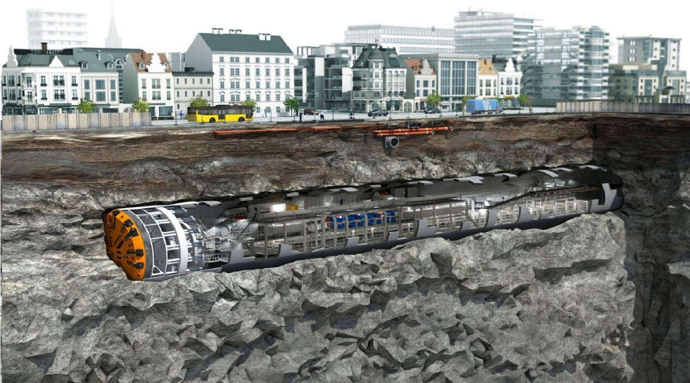
Photo Source: National Geographic, Tunnel Boring Machine
