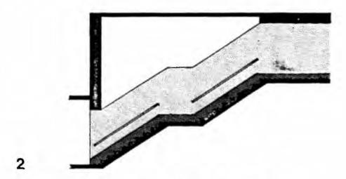
All exposed walls on stairways are to be painted with heavy duty paint or approved synthetic coating.
