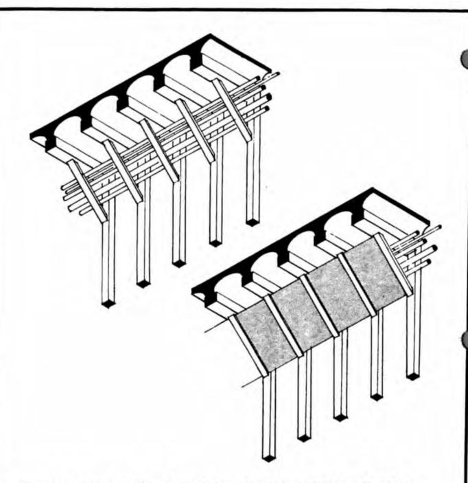
Cover up exposed runs of conduit, wherever possible, in neat new ducts or chases. When this is not possible, design new conduit and relocate.
