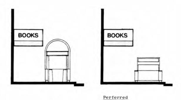
Building projections - existing signs, lights, and similar elements should be considered when selecting the surface structure. Close proximity or actual contact of MBTA structures with nearby elements should be avoided.
