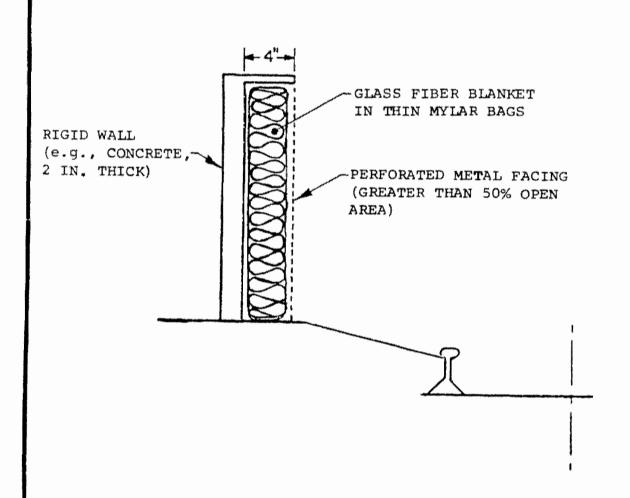
SCHEMATIC DIAGRAM OF BARRIER CONSTRUCTION
