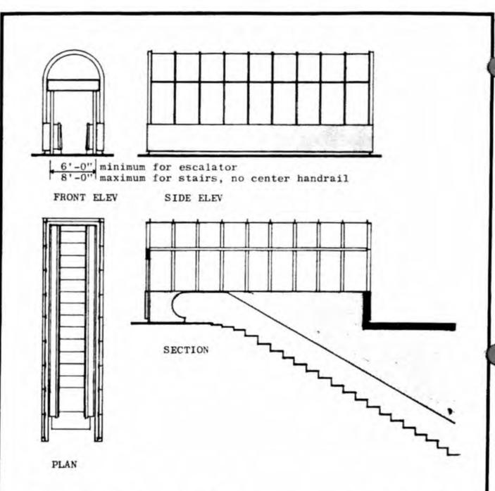
The Type 1 steel and glass structure permits maximum visibility of the surrounding area and also permits maximum light penetration to the lower level, while providing complete weather protection.
