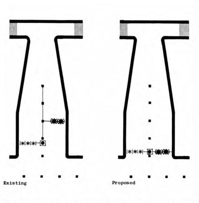
Simplify circulation spaces by eliminating and relocating barriers.
