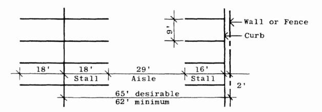
Ninety degree parking is preferred with angle parking used only where space is restricted. The preferred dimensions for right-angle parking bays are shown above.
