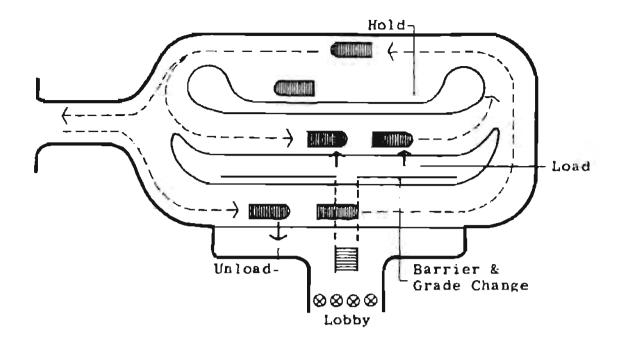
The scheme above involves intensive use of loading berths by many routes in a random manner. It requires a large platform for waiting passengers, an audio/visual system, and a traffic controller for identifying buses. This scheme offers short walking distances, but is more hectic for the rider due to the constant milling about on the platform. Buses may layover in the hold area in this scheme.
