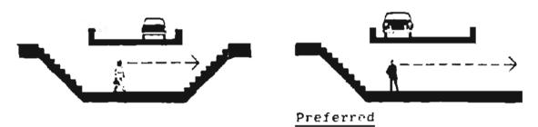
If possible, pedestrian overpasses or underpasses should be used where one end can be at or near grade. This minimizes the successive up and down movements, allows better surveillance, gives the pedestrian a sense of orientation, and is generally more pleasant.
