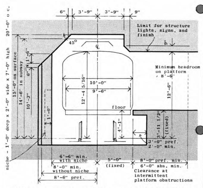
Clearances shown are for new facilities. Existing clearances and absolute minimum clearances for special conditions must be obtained from the MBTA. Track and platform alignment and profile is determined by the engineers in conjunction with the Station Architects and the MBTA. For platform widths see Part IV Components. Structural dimensions shown are minimum unless otherwise noted.
