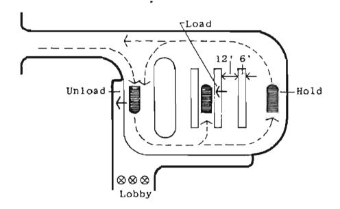
When space does not permit use of long in-line loading areas, a more compact arrangement, utilizing small island platforms, may be used. This system, however, leads to uncontrolled pedestrian crossings over a large part of the busway, and hence increased danger and possible movement delay.
