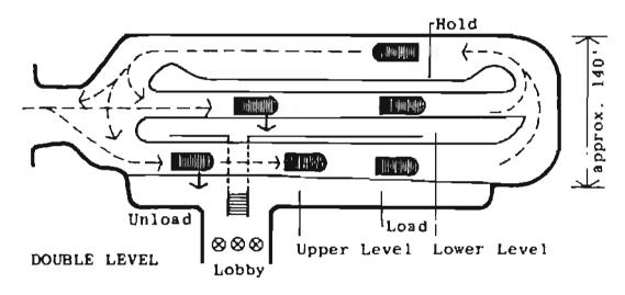
With the above scheme, the number of loading berths may be reduced by having buses layover in the hold area and stop in the loading berths just long enough to load. More routes can double up at a single berth this way.
