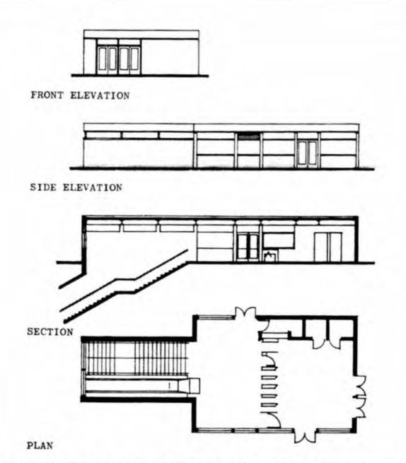
The Control House Type differs from the purely entrance and exit surface structures by the inclusion of a fare collection area. The dimensional recommendations contained in the section on fare collection apply.
