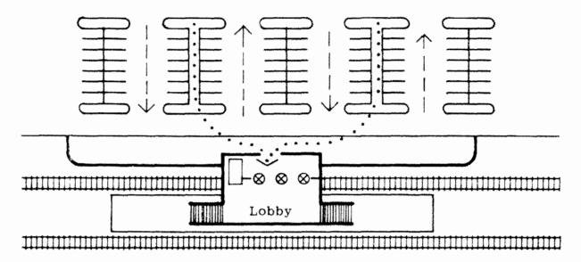
Circulation within the parking bays should be one way, with a counter-clockwise pattern preferred. Entrys to bays and the roadway system should be well signed. Bays should be aimed toward the station entry so that pedestrians flow along the bays to the station. Crosswalks at busways should be marked.
