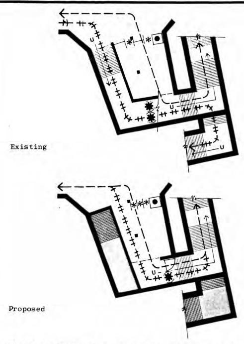
Clarify circulation by eliminating useless options, and where space is adequate, by combining entrance and exit circulation.
