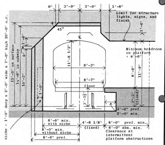
Clearances shown are for new facilities. Existing clearances, and absolute minimum clearances for special conditions must be obtained from the MBTA. Track and platform alignment and profile is determined by the engineers in conjunction with the Station Architects and the MBTA. For platform widths see Part IV Components. Structural dimensions shown are minimum unless otherwise noted.
