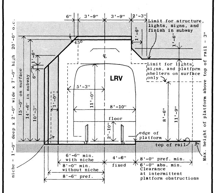
Clearances shown are for new facilities. Existing clearances, and absolute minimum clearances for special conditions must be obtained from the MBTA. Track and platform alignment and profiles are determined by the engineers in conjunction with the Station Architects and the MBTA. For platform widths see Part IV Components. Structural dimensions shown are minimum unless otherwise noted.
