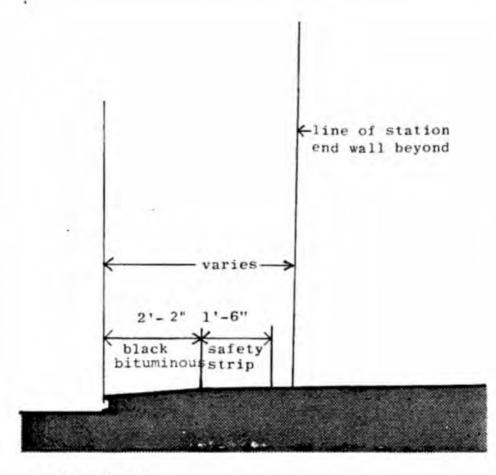
Safety Strip Material : Heavy-duty abrasive coating
