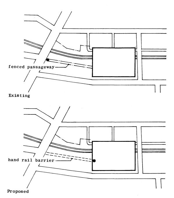
Eliminate unnecessary barriers that have unpleasant visual and psychological effects. In this case relocation of the exit gate makes possible the replacement of a fenced passageway with a hand rail safety barrier.
