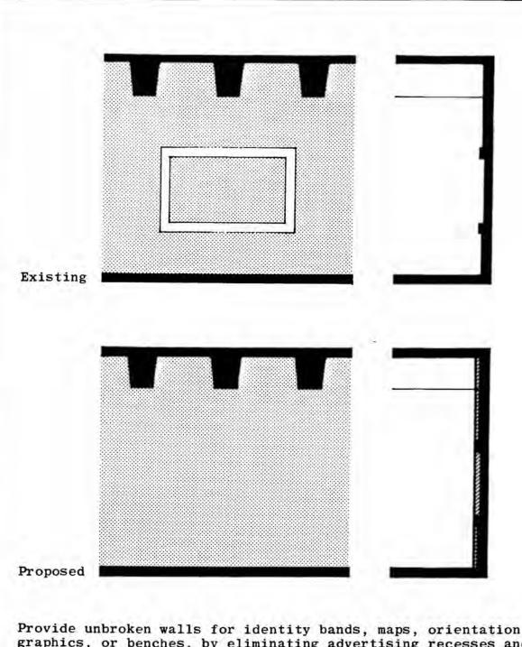
Provide unbroken walls for identity bands, maps, orientation graphics, or benches, by eliminating advertising recesses and other miscellaneous changes of plane.
