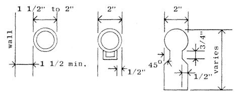
h. The handrail must be stainless steel or hardwood. The supporting structure may be stainless steel or black painted galvanized steel. All pipe rail joints must be welded and ground smooth.
