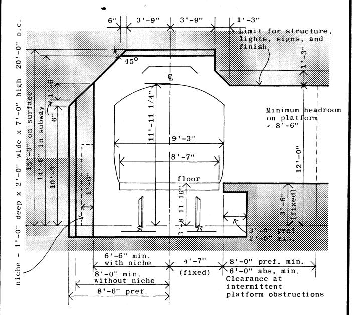
Clearances shown are for new facilities. Existing clearances, and absolute minimum clearances for special conditions must be obtained from the MBTA. Track and platform alignment and profile is determined by the engineers in conjunction with the Station Architects and the MBTA. For platform widths see Part IV Components. Structural dimensions shown are minimum unless otherwise noted.
