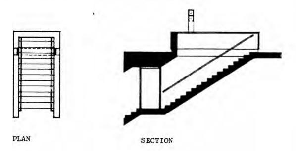
The Type 2 structure provides access to stations by means of a minimal surface structure. It should be used where the vaulted type would result in a physical or visual interference with surrounding elements.
