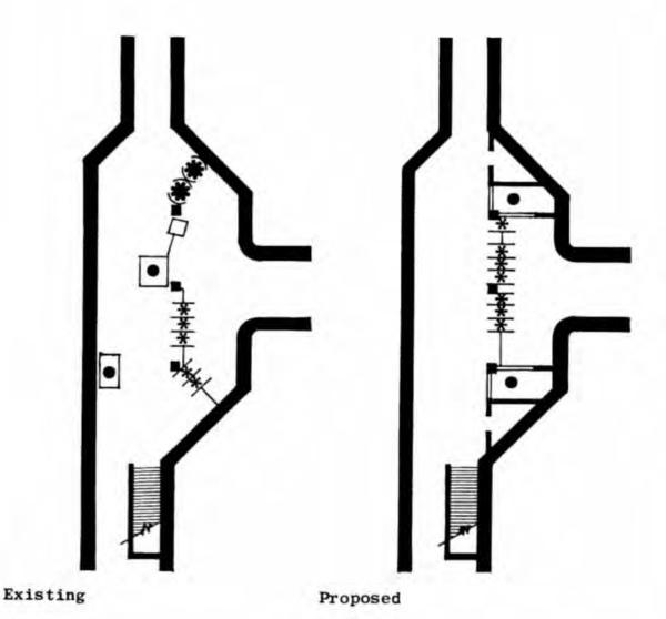
Build-in components, such as change booths, to relate to structure, where appropriate. Reduce clutter in confined areas.
