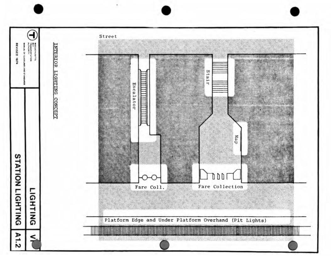
The type of lighting and the light intensity will be determined by the function of the area.
