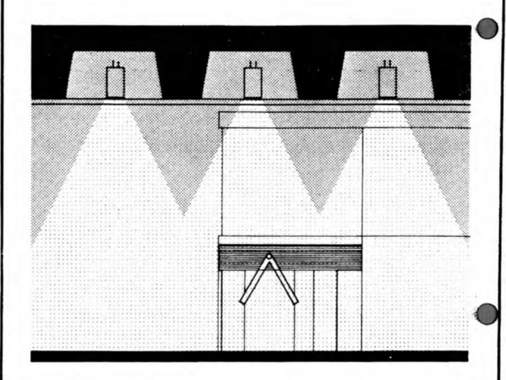
Raceway - supported High Intensity Discharge downlights.
