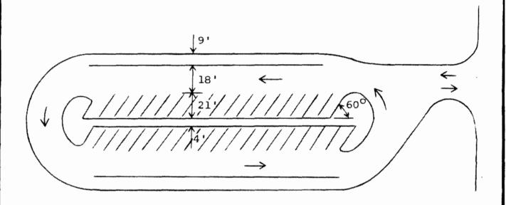
Curve radii and roadway widths should be sufficient to permit operation of buses in the kiss-and-ride area if required.
