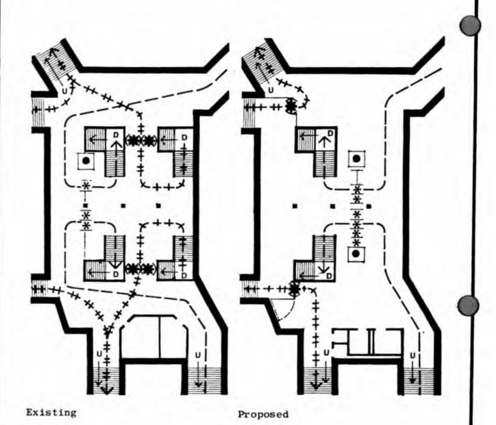
Improve circulation by providing adequate space to eliminate bottlenecks.
