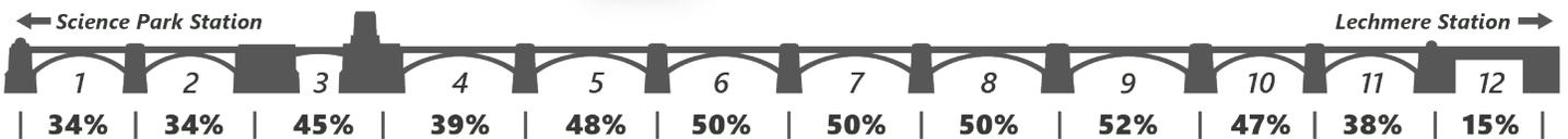
1,700 ft of Structural Repairs Underway (12 Spans)
